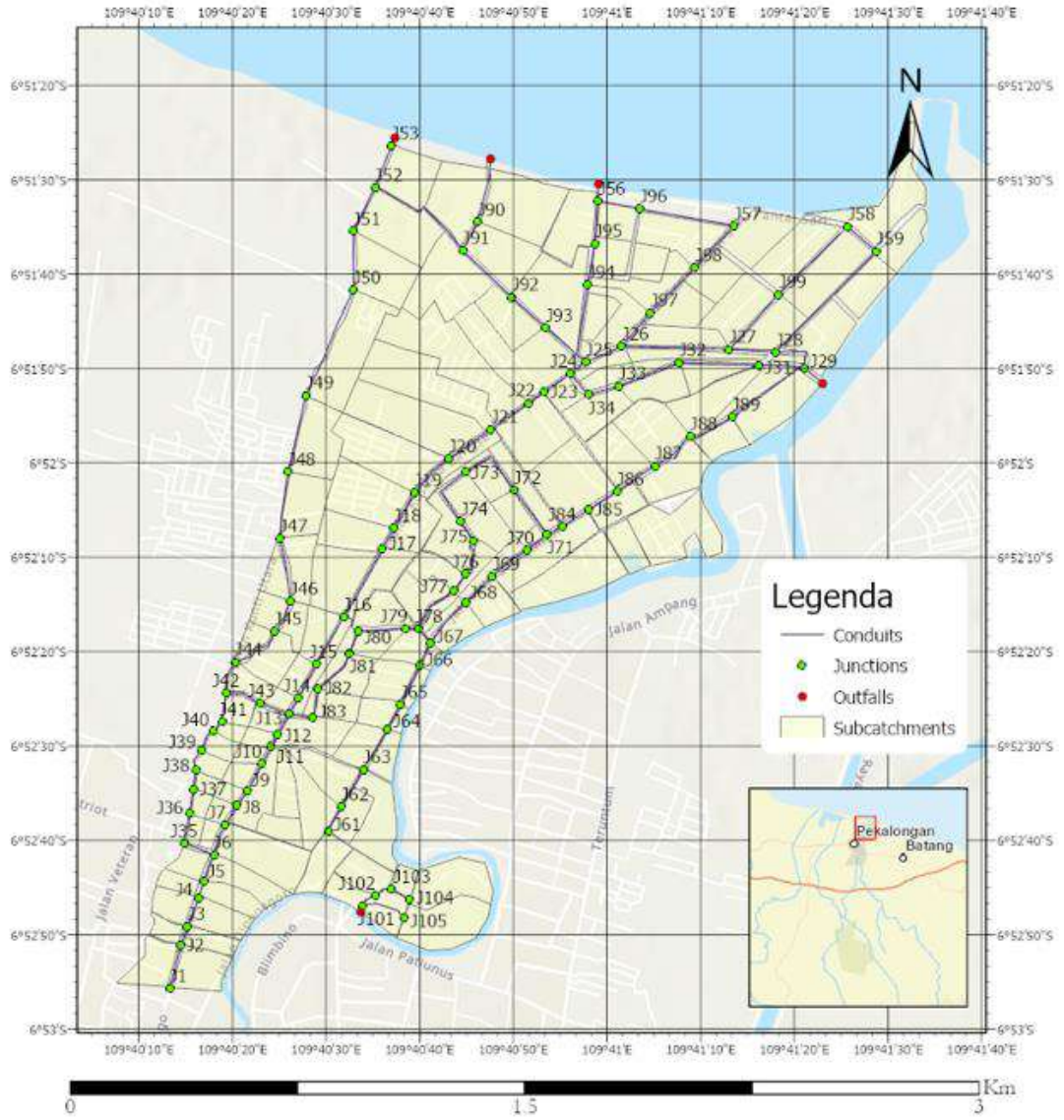
Gambar 4. 21 Skema Drainase dan Subcacthment Loji
